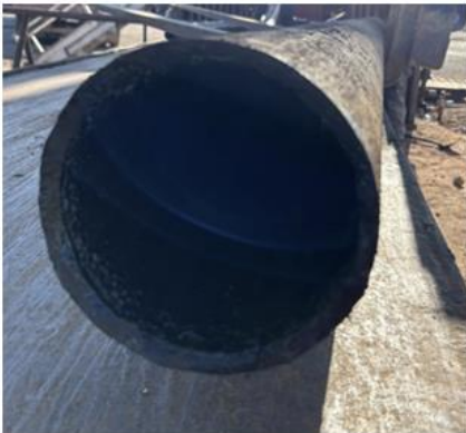
6 3/8" CSG 0.31" wall cut using a 3" CPC (6/2024)
