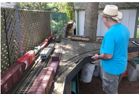
Where real estate allows, a wye offers so much more than just turning an engine. Operators can turn an entire train if the trackwork beyond the three legs of the wye junction is long enough.
