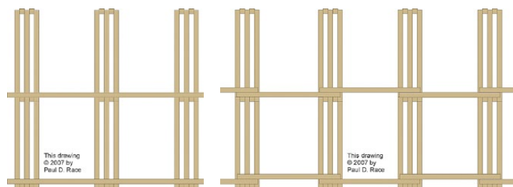
Using a single piece of wood for the crossbars simplifies construction.
