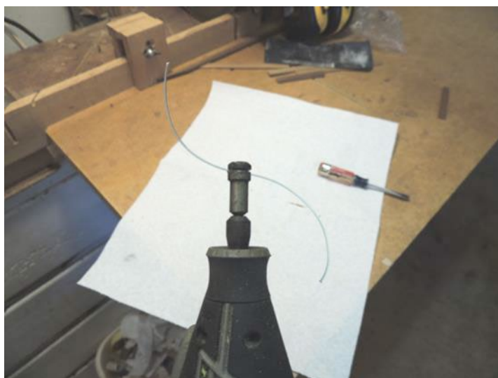
Use a simple overhand knot (shown in the top photo) to tie the line around the spindle screw, tighten the screw down, and you are ready for trimming.
