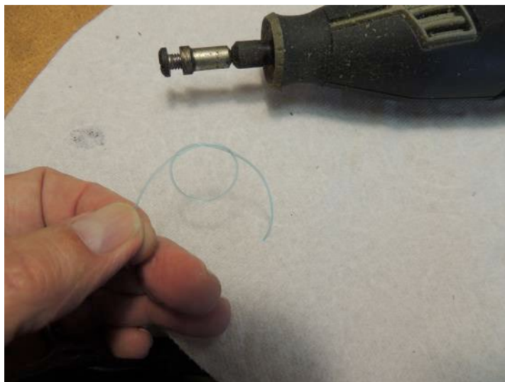
Dremel Model 8220 with a mandrel from a Harbor Freight rotary tool accessories pack. The mandrel is larger in diameter than the standard Dremel mandrel and provides a better holding surface for the 60# fishing line I found in my tackle box.
