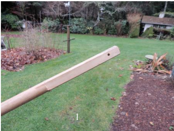
An old broom handle drilled and cut to hold the block of wood.
