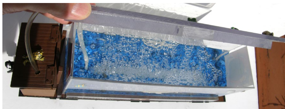
Aerator in operation; Note tubing requires a drilled hole in the cover.
