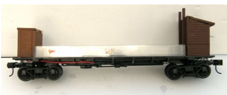
Metal-wheel flat car with battery & electronics boxes at ends. Aquarium tank fits into clear plastic frame.
