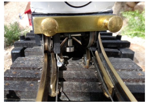
Wheels, cable hook and control magnet passing through lower ABT Switch. Hook and magnet placement must be precise.
