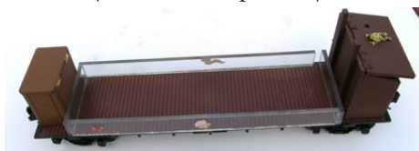
Metal-wheel flat car with battery & electronics boxes at ends. Aquarium tank fits into clear plastic frame.
