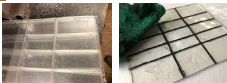
Grooved acrylic, painted muntins & mullions, and painted aluminum angle combine to create windows.
