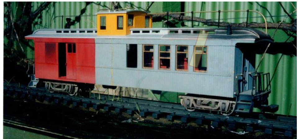
Mike's first LGB chop D&RGW Combine 215 made from one and a half LGB combines. The other half was added to an LGB coach.
