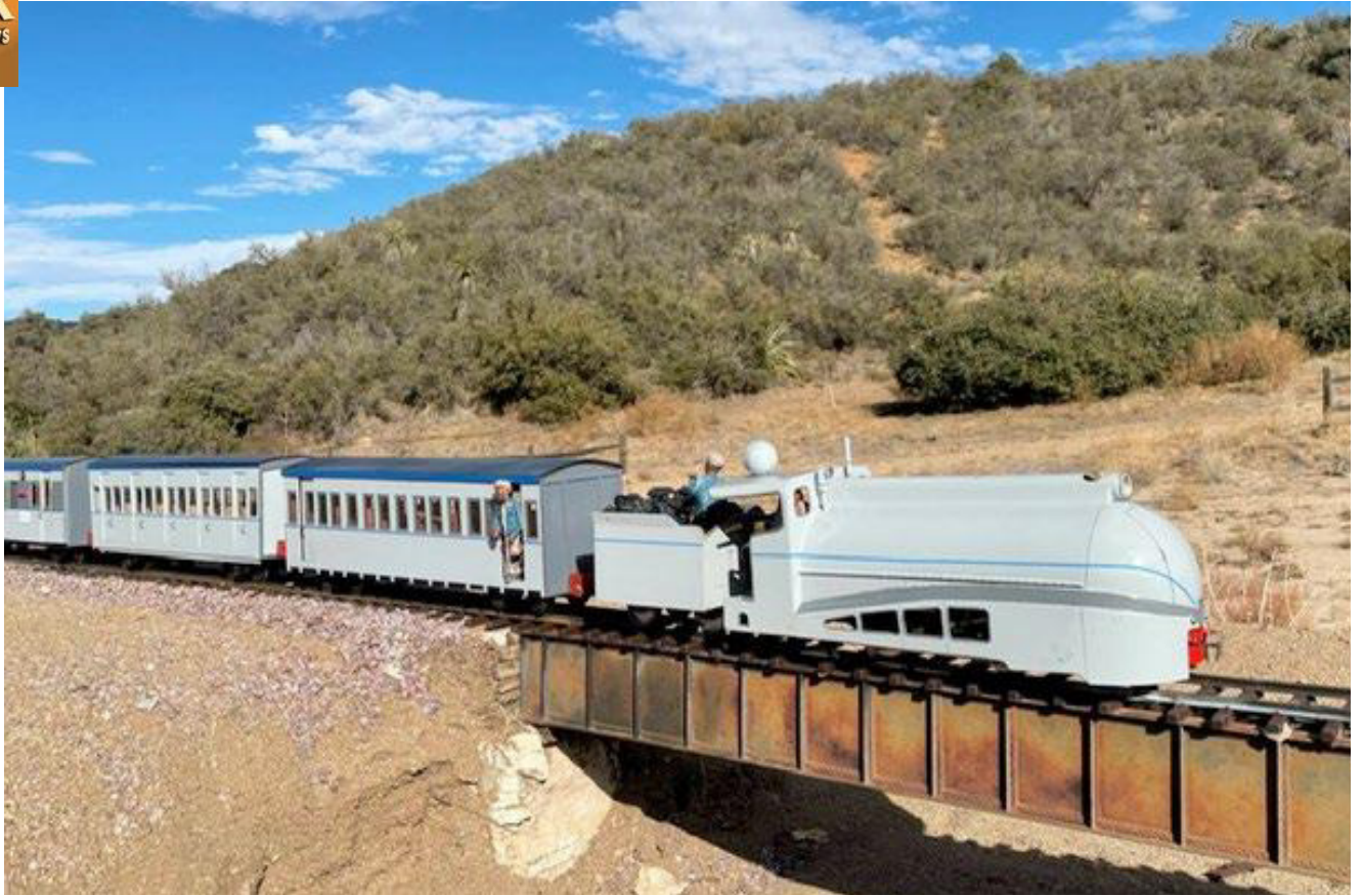
Above: Pete Comley built this "streamlined" version of a Darjeeling B locomotive with 1930s coaches used very briefly on the Darjeeling Himalayan Railway. The 1:19 scale model shell sits over a Roundhouse Darjeeling class B chassis with the gas tank in the tender. • San Jacinto & Santa Rosa Mountains, California
