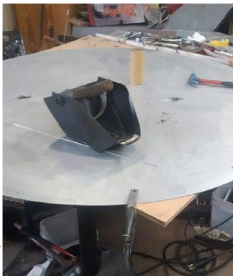
Daniel Peck of Daniel Custom Products built the turntable, starting by cutting a 5 foot aluminum disk.
