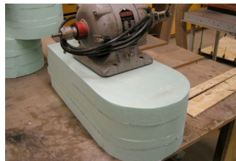
Fig. 2: Arch glue-up pressed together. (Motor used for weight)
