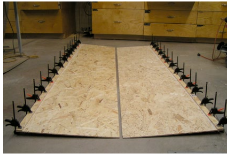
Fig. 4: Gluing strip for wall notch to the OSB form
