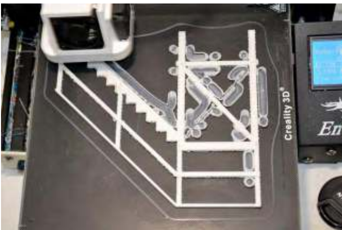
Above - The first few layers of the stairway print. Nozzle 0.4mm, 205C, Bed 60C, Speed 80mm/sec, Layer height 1.2mm.
