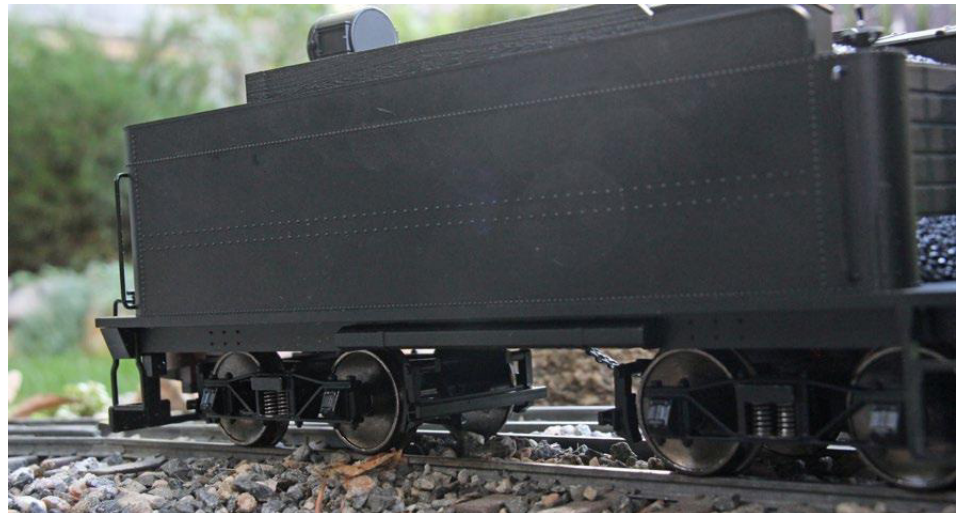
A poling pole (for moving cars on adjacent tracks) is cast into the engineer's side of the tender frame just above the wheels.
