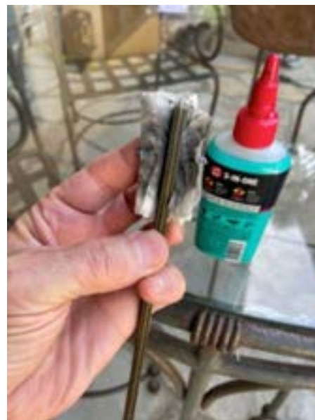
(Above) Oiling rail pre-threading.
