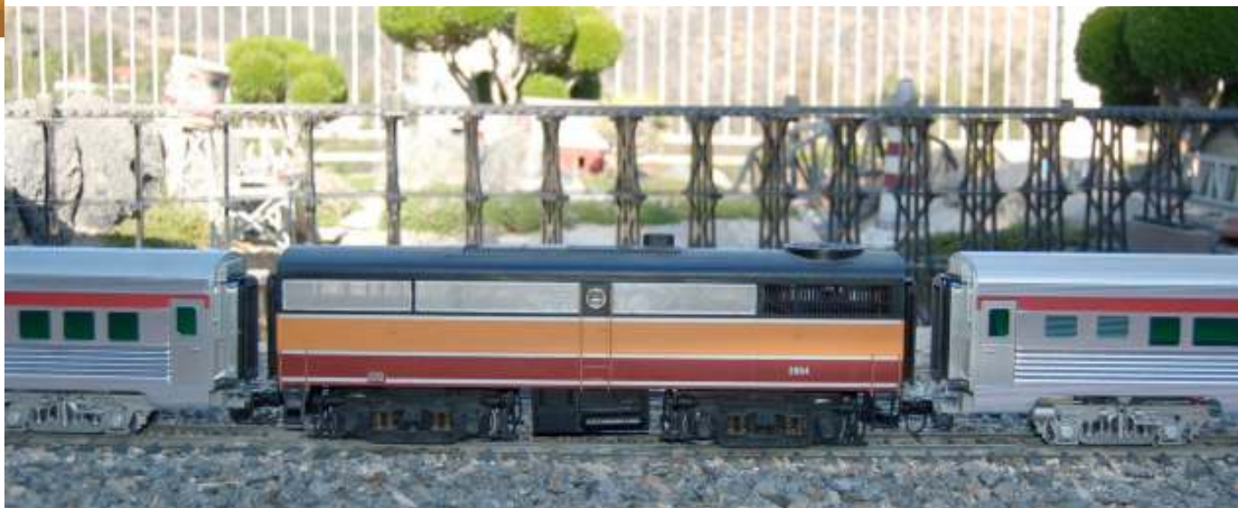
The lowered height of the modified coach on the left allows it to sit more realistically when pulled by this AristoCraft FA/FB unit.
