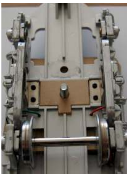
Testing position of truck centering insert in place on truck mounted coupler before final reassembly.
