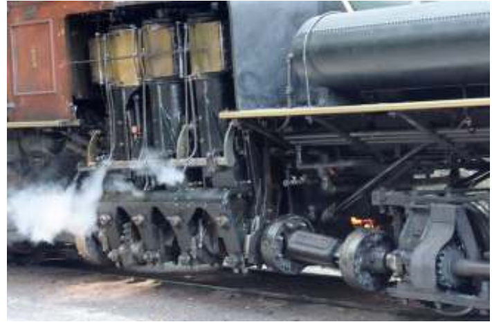
The Roaring Camp and Big Trees Railroad. In the middle of a grove, the two-truck Shay "Dixiana" backed up, gathered steam, and gave us all a dramatic run-by. She achieved speeds in excess of 16 mph. On the right, the Shay's hard-working cylinders, crankshaft and drive shafts.
