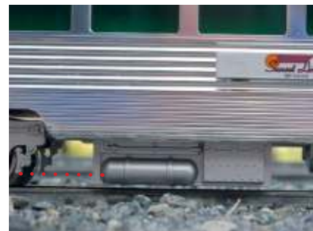
Modified. The bottom of the air tank is well below the brake assembly.
