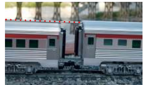
Modified coach (left) sits lower on its trucks for an overall reduction in height.
