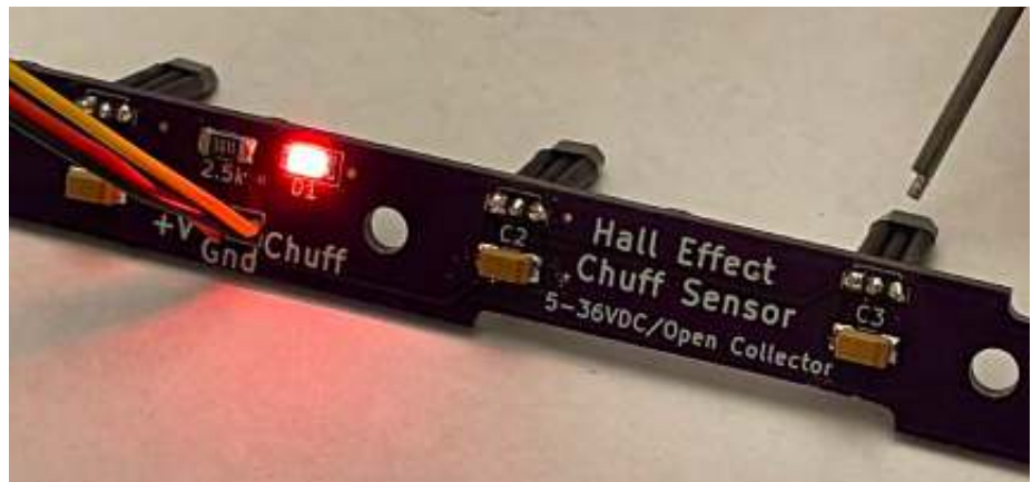
Eric Timberlake's custom made Hall Effect Chuff Sensor Board wired to test fire using magnet on rod upper right.
