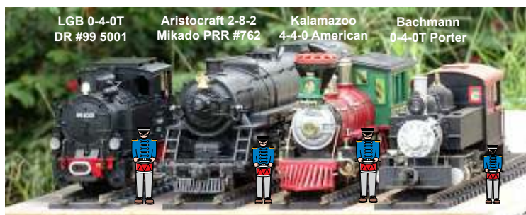
1:22.5 Scale. Correct for European meter gauge. 1:29 Scale. Slightly oversized for standard gauge. 1:24 Scale. Slightly undersized for 3-foot gauge. Correct for 42" gauge. 1:32 Scale. Correct for standard gauge.
