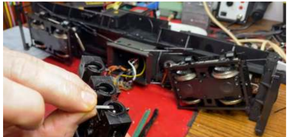
Testing placement of Hall Effect Sensor DRV5033 above micro-magnet glued to top of cylinder rod.
