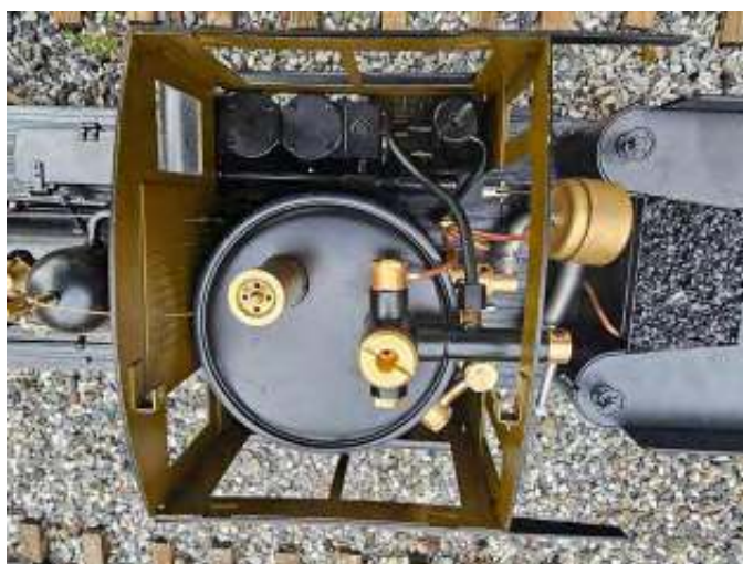
The large boiler hidden in the cab.
