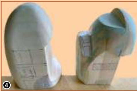
The front and rear of the train have complicated shapes, so I made those from basswood and finished with Bondo to make a smooth paintable surface (photos 4 & 5).
