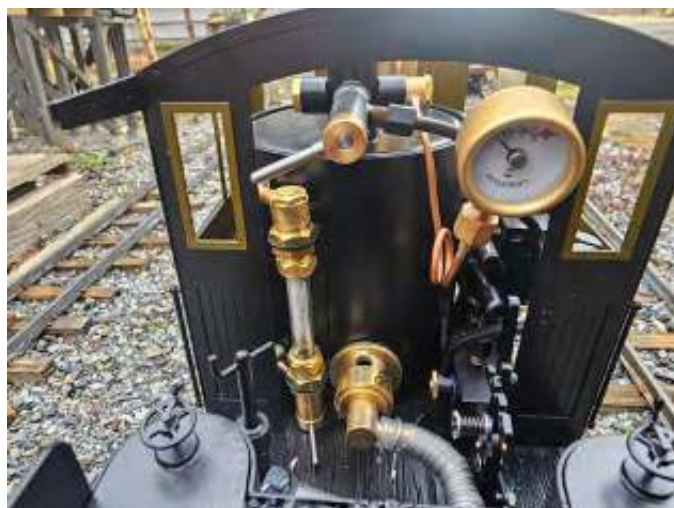
The pressure gauge and sight glass are easily readable. The sight glass has a blow-down valve.
