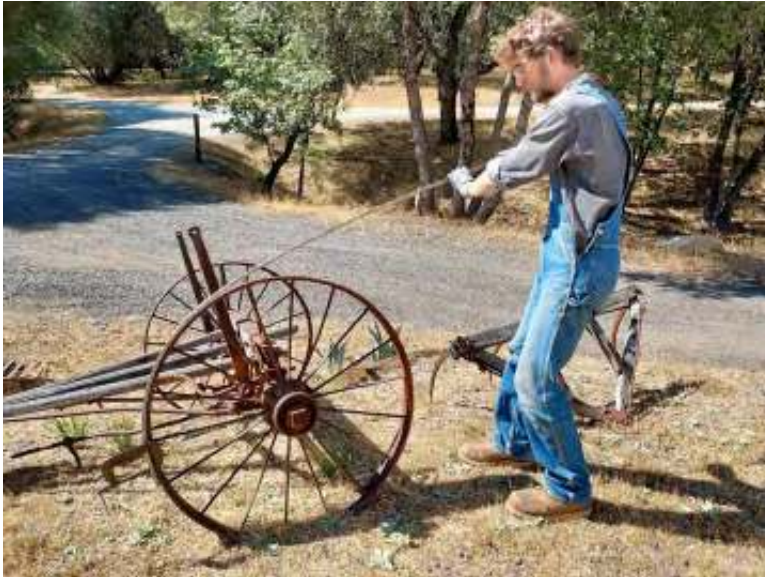
Photo 2 Unorthodox method of bending the tubing.
