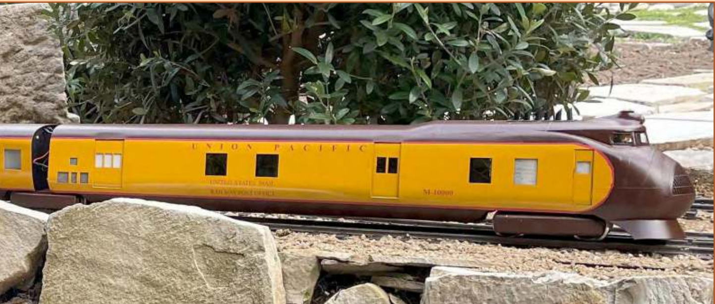
The front and rear of the train have complicated shapes, so I made those from basswood and finished with Bondo to make a smooth paintable surface (photos 4 & 5).
