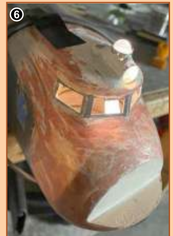
The front and rear of the train have complicated shapes, so I made those from basswood and finished with Bondo to make a smooth paintable surface (photos 4 & 5).
