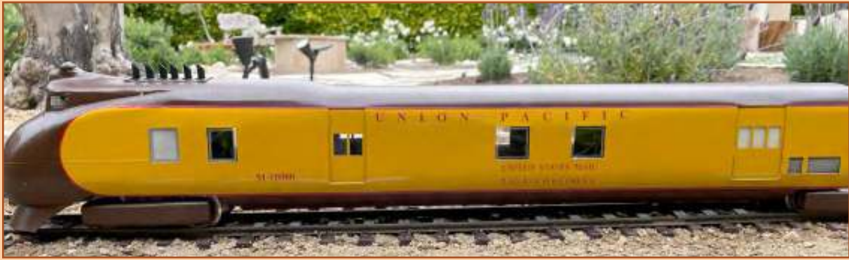
A USA Trains power block drives the front truck and 14.4V Li-ion batteries give well over an hour of running time.
