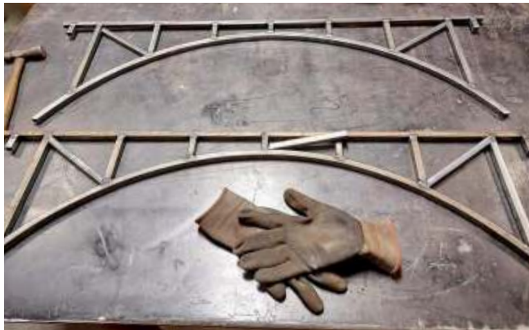
Photo 7 Fitting the cross braces.
