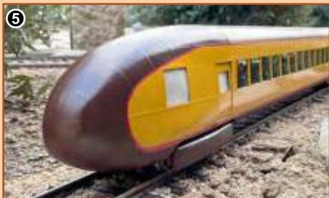
The headlight and famous vertical searchlight were made from glass balls with an LED to light them (photo 6). All the cars have interior LED lighting which makes for great night running. The distinctive and delicate front grille was expertly made as a 3D print by my colleague Chris Coley and gives the final touch to the project.
