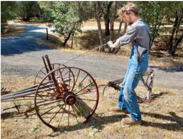
Photo 2 Unorthodox method of bending the tubing.
