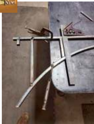
Photo 5 Using a carpenter's square to line everything up. Note the tack welds.
