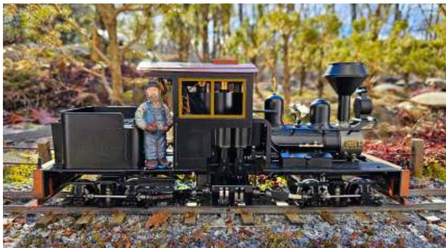
The Shay on the Kittatiny Mountain Railroad. A water bath around the gas tank in the tender helps cool weather running.
