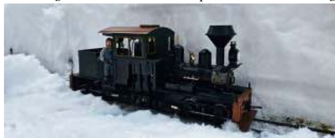
The Shay on the Kittatiny Mountain Railroad. A water bath around the gas tank in the tender helps cool weather running.
