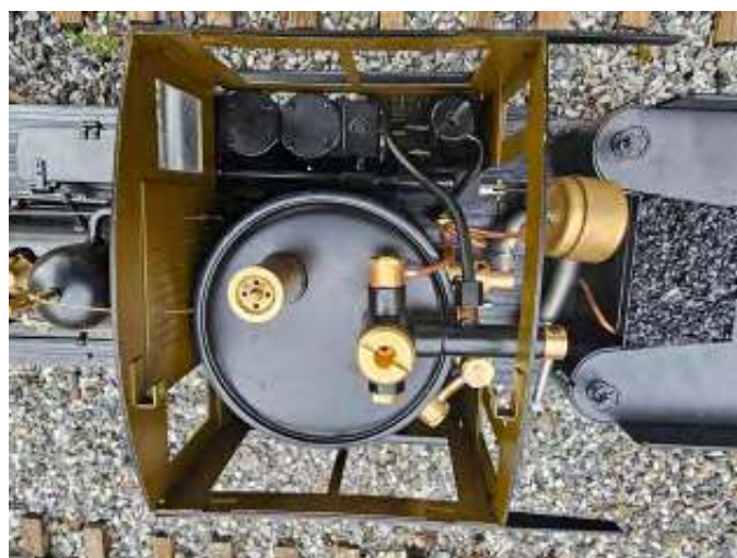
The large boiler hidden in the cab.
