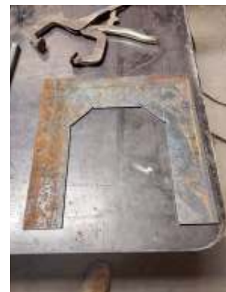
Photo 4 The cut-out backing plate.
