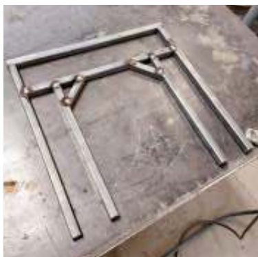
Photo 6 Assembling the frame.
