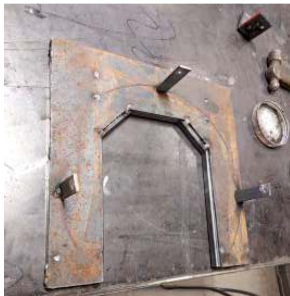
Photo 9 Welding mounting tabs on.
