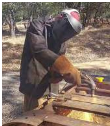
Photo 3 Using a plasma cutter.
