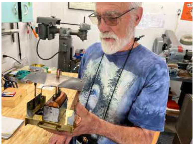
Craig shows a Denver oscillating cylinder live steamer that he was building from a Marc Horovitz design.
