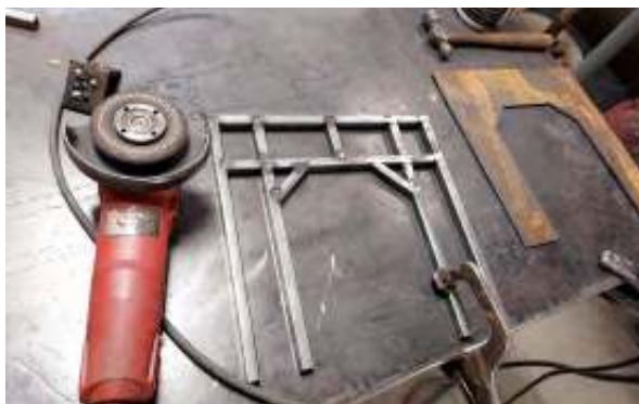
Photo 7 Grinding the welds flat on the back of the frame.
