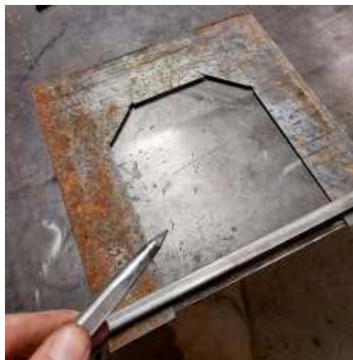
Photo 5 Scribing board lines to simulate wood.
