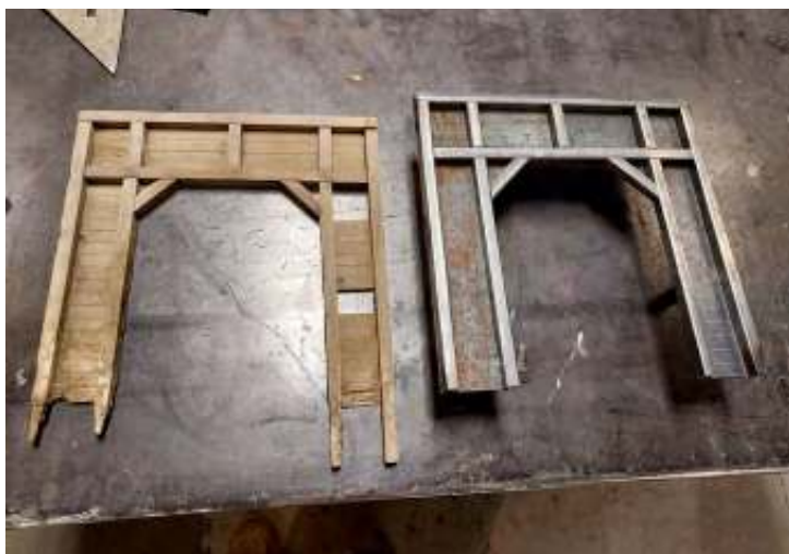
Old timber portal, New steel portal.
