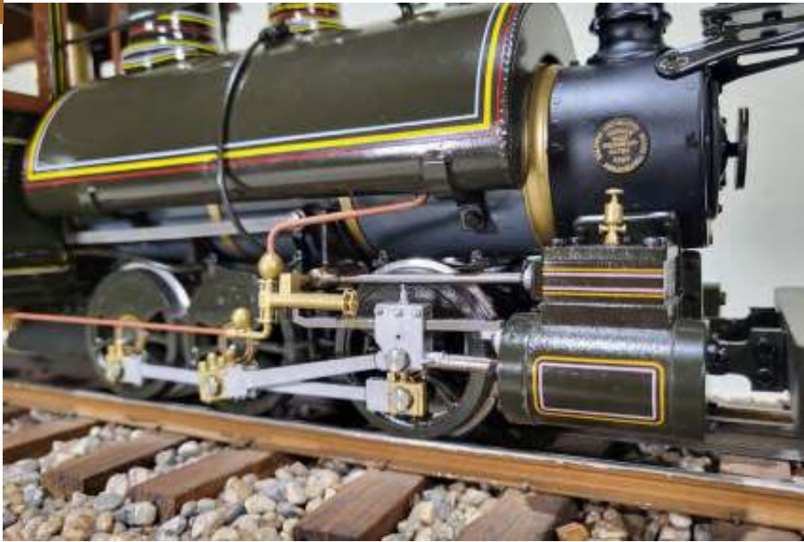
Efficient slide valve cylinders with a 1/2" bore drive a full working Stephenson valve gear.
