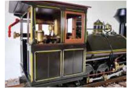
Throttle behind cab is easily accessible.
