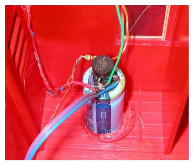
The green and orange wires that come off of the capacitor in the photo above go to the roof LEDs. The two wires that are twisted together on the left go to small 3mm LEDs that were inserted into the bottom of the side lanterns on the caboose as seen below. They are quite bright as you can see in the opening photo of the caboose at night.
