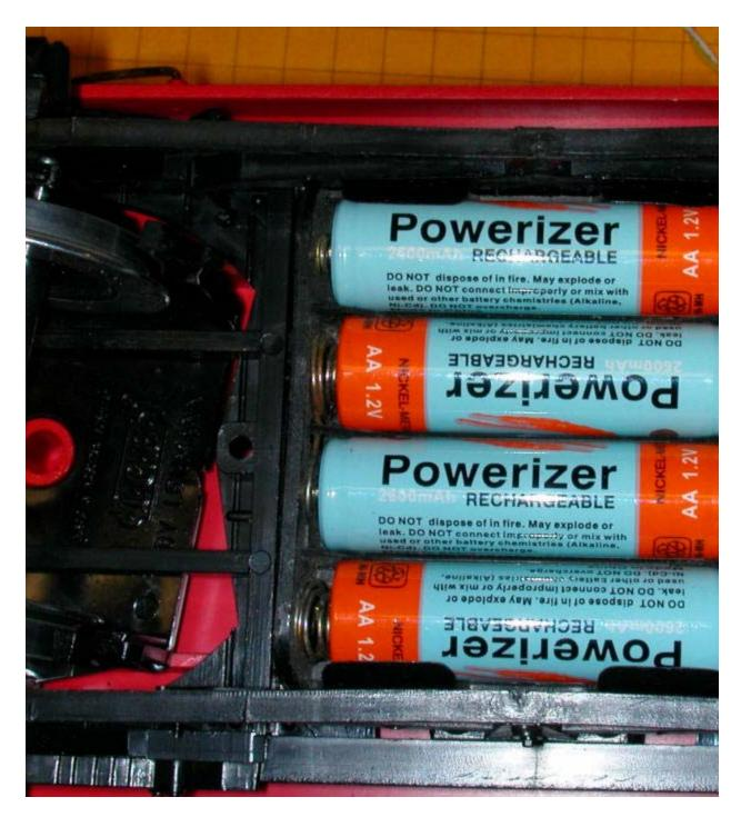
If your car does not provide enough space for a battery holder and 4 AA cells as in the photo above, NiMH cells are also available with solder tabs so that you can make a smaller battery pack by soldering cells together.
