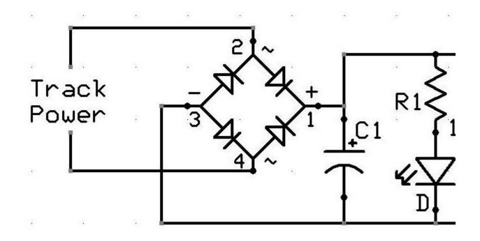
The photo below shows the circuit above. The track power comes through the wires on the left. The output of the bridge rectifier is connected to the capacitor and then to a positive bus (lower wire) and a negative bus (upper wire). The four LEDs and their four current limiting resistors are connected between the positive and negative leads.
