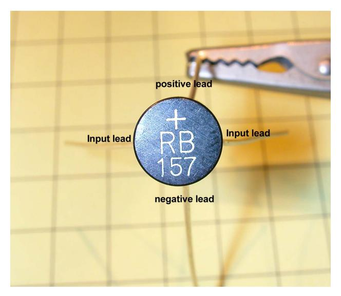
You will also note that the positive lead on bridge rectifiers is generally longer than the other three. The size difference between the bridge rectifiers in the sample is due to their current handling capacity. The largest is rated at 3 amps and the smallest at 1 amp. LEDs draw so little power that any size bridge rectifier is likely to suffice.
