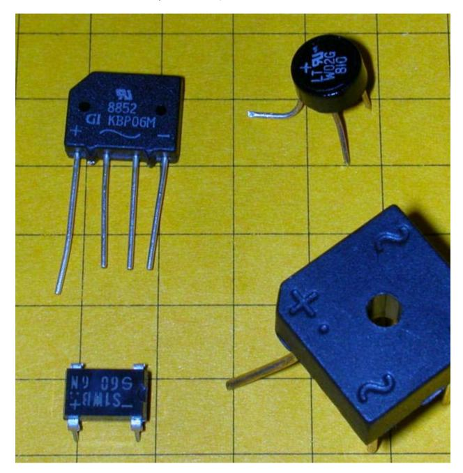
Bridge rectifiers have two input pins (frequently marked with the symbol for alternating current "~") and two output pins that always provide a positive and a negative terminal no matter what the polarity may be on the input terminals. The input pins go to the track pickups and the output pins go to the LED(s).
