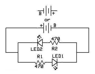
If LED1 is the locomotive's headlight it will light only when the train goes forward. If LED2 is a rear facing spotlight, as we see on some tenders, it will only light when the train is going backwards. Is it necessary to have both LEDs in the circuit? The answer is no. To have just a headlight work when the engine is going forward remove LED2 and resistor R2 from the circuit.
