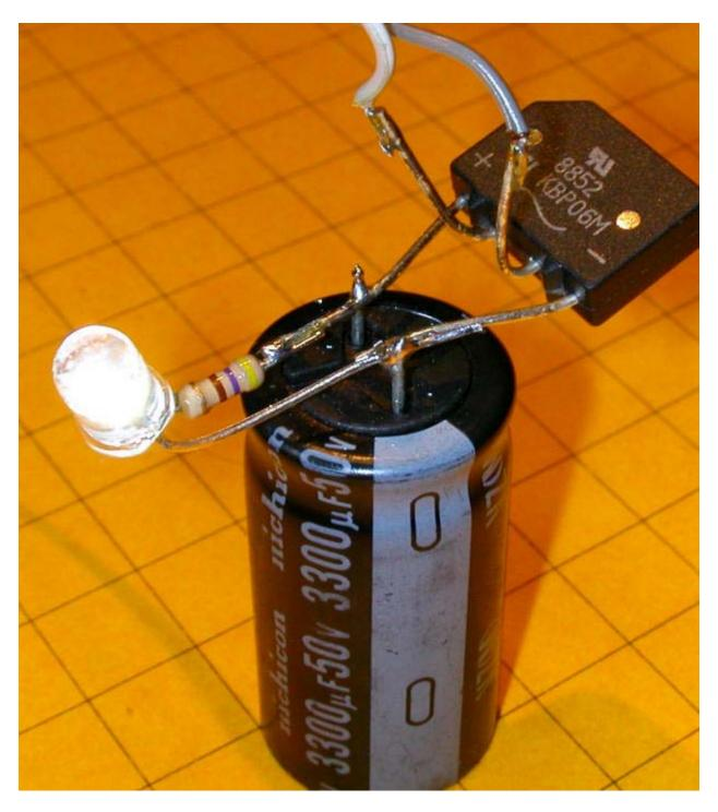
Additional LEDs can be added by wiring them in parallel as shown here.
