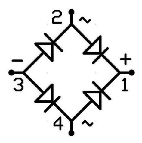
The voltage of unknown or varying polarity goes into pins 2 and 4 and the output is on pins 1 and 3. The only significant drawback to using a bridge rectifier in a circuit is that the output voltage is about a volt lower than the input voltage. Keep in mind that you can make a bridge rectifier from four diodes by wiring them as in the illustration above. I have done this on a number of occasions when I didn't have a bridge rectifier on hand or when I needed a particularly small unit.
