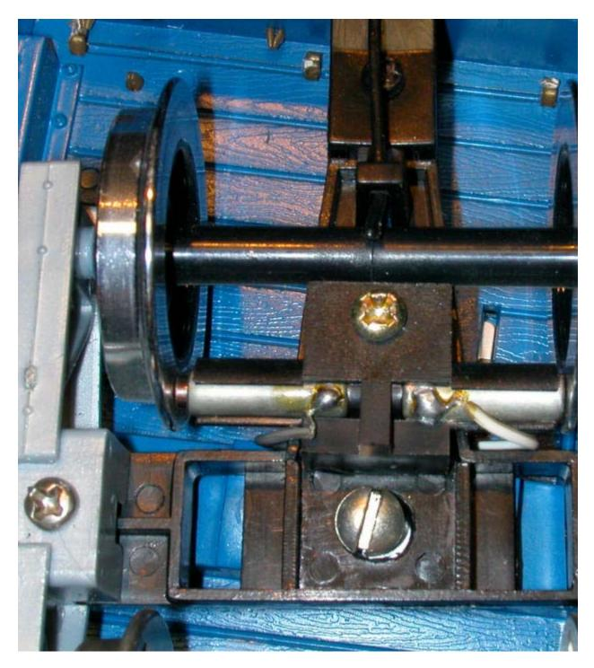
The two wires from the track pickups are routed through a hole in the car's floor and connected to the input terminals on the bridge rectifier. The output terminals go to the LED circuit.
