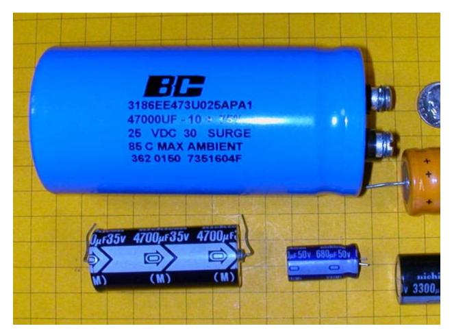
The capacitors in the photo above range from 680 uF @ 50 volts (bottom center) to 47,000 uF @ 25 volts in the upper left. Note that the large blue capacitor is rated at only 25 volts and may not be adequate if you tend to run your trains at full voltage.
