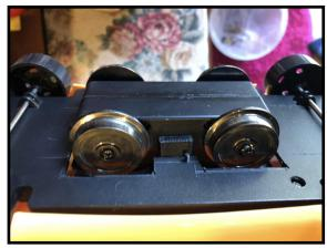
Originally it was an Aristocraft FA/Eggliner motor block. And he cut a square hole in the chassis and bolted it in. For the other vehicles he 3D printed some very basic axle mounts and glued them on.
