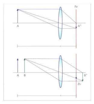
A correctly focused object (A) leads to a sharp image on the film/sensor plane (A"). An object which is closer (B) would be sharp behind the film/sensor plane (B"). The image point of the top of the object is not exactly focused as a point, but as a so-called circle of confusion. If this exceeds a certain size, we perceive the images being blurred.
