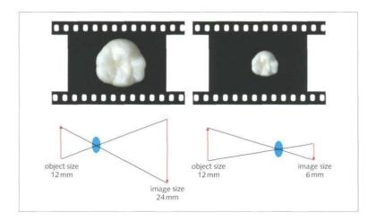
For practical reasons, the magnification ratio may be referred to 35-mm film format. If the frame includes a distance of 36 mm, we speak of a magnification ratio of 1:1. If a full frame includes 18 mm, we are speaking of a magnification ratio of 2:1. In dental photography the following reproduction ratios are important (approximate):
