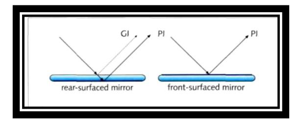
Rear-surfaced mirrors provide a primary image (PI) from the back reflective surface, but also a secondary image from reflection off the front glass surface ("ghost image" = 01). Such mirrors are inexpensive, but not suitable for our purposes.
