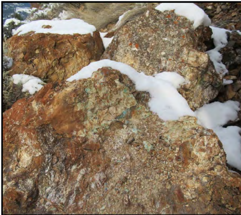
Photo 6: Malachite-copper stained iron breccia boulders from old open-cut/pit (photo 4). Alteration minerals include brecciated quartz, calcite, iron carbonate –dolomitic (ankerite/siderite), includes kaolinitic and cryptocrystalline-like agate mineral fragments.
