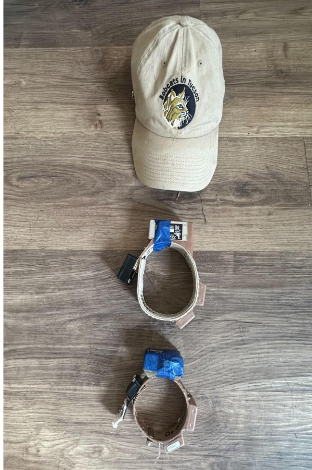
Figure 7. Telonics TGW-4277 (top) and TGW-4177 (bottom) radio collars
