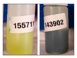
Figure 2: New fluid and used fluid sample
