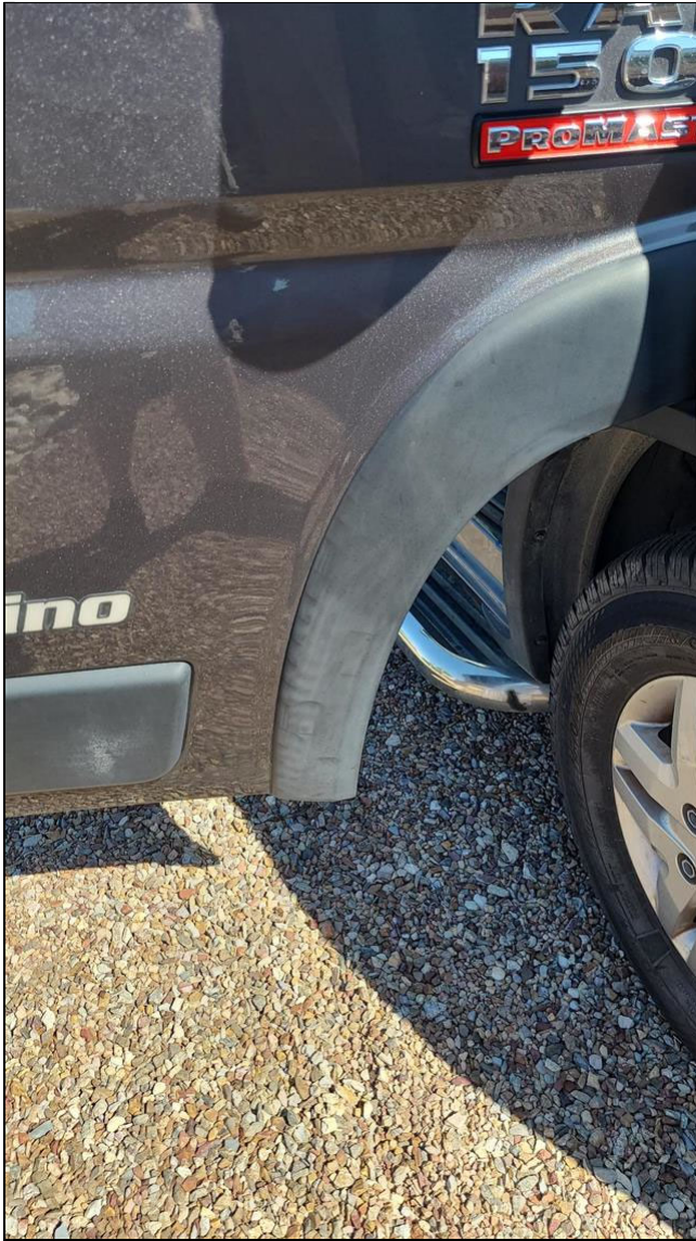
Oxidation on Wheel Well
