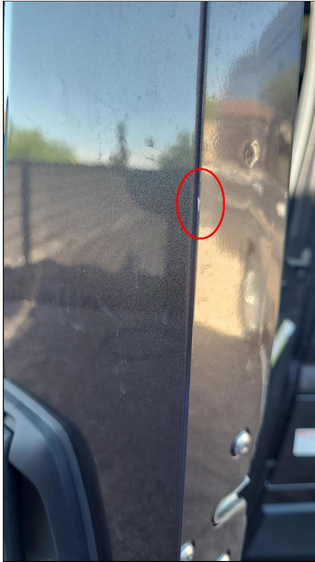
Chip in Paint on Door Edge
