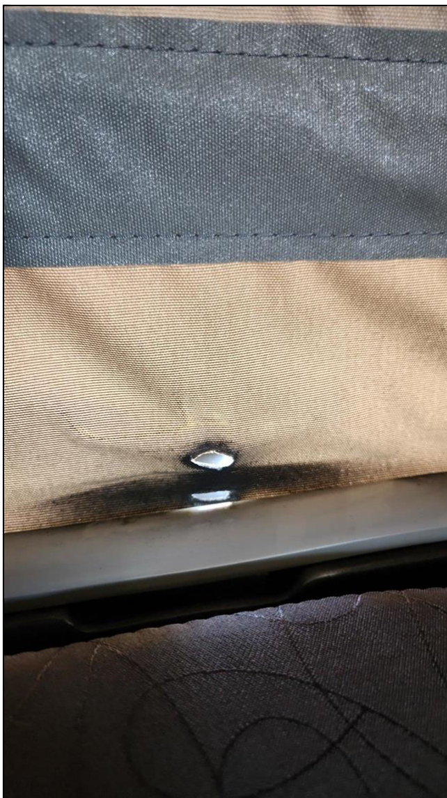
Wear Hole in Canopy
