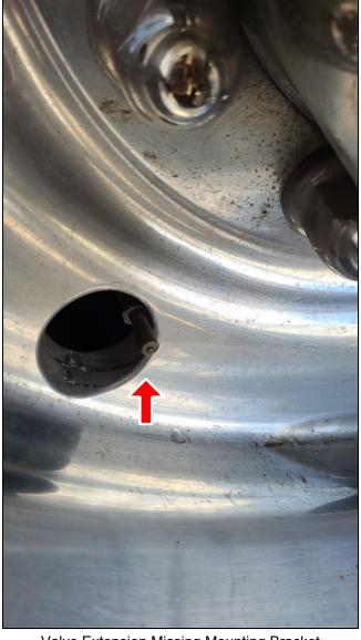
Valve Extension Missing Mounting Bracket
