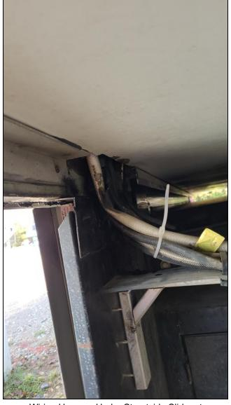
Wiring Harness Under Streetside Slideout
