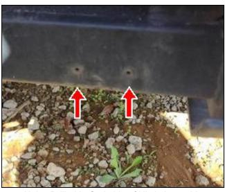
Holes Drilled in Curbside of Hitch Assembly
