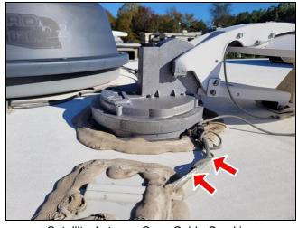
Satellite Antenna Coax Cable Cracking
