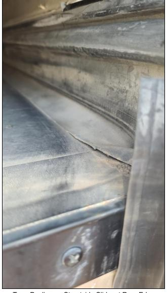
Tape Peeling on Streetside Slideout Rear Edge
