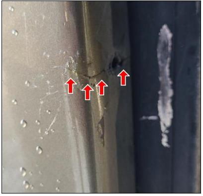
Crack in Streetside Sidewall
