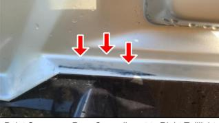
Paint Scrape on Rear Capwall next to Right Taillight
