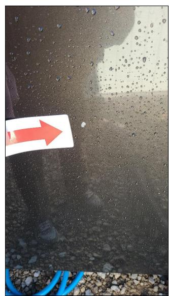
Three Chip in Paint on Front Edge of Door
