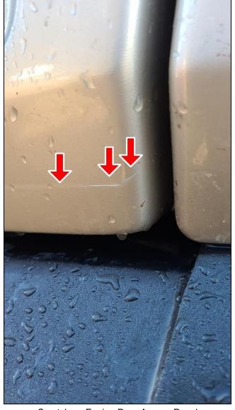
Scratch on Engine Door Access Panel
