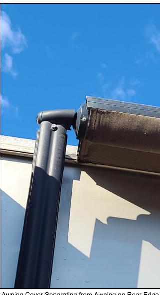
Awning Cover Separating from Awning on Front Edge Awning Cover Separating from Awning on Rear Edge
