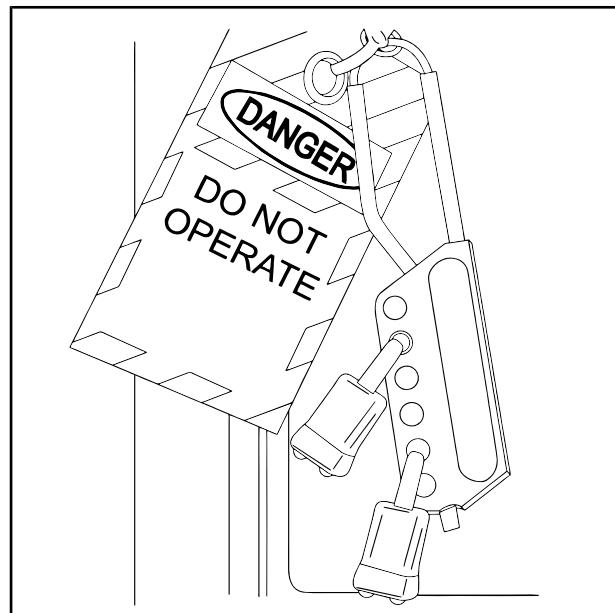
Fig.2-16 Lockout/tagout alert tag
