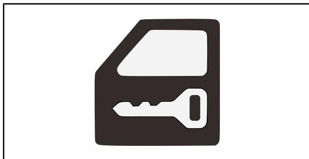
Fig.3-58 Door switch indicator light
