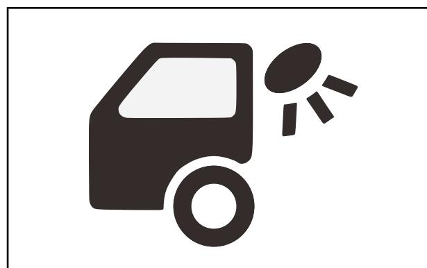
Fig.3-89 Working lamp indicator light
