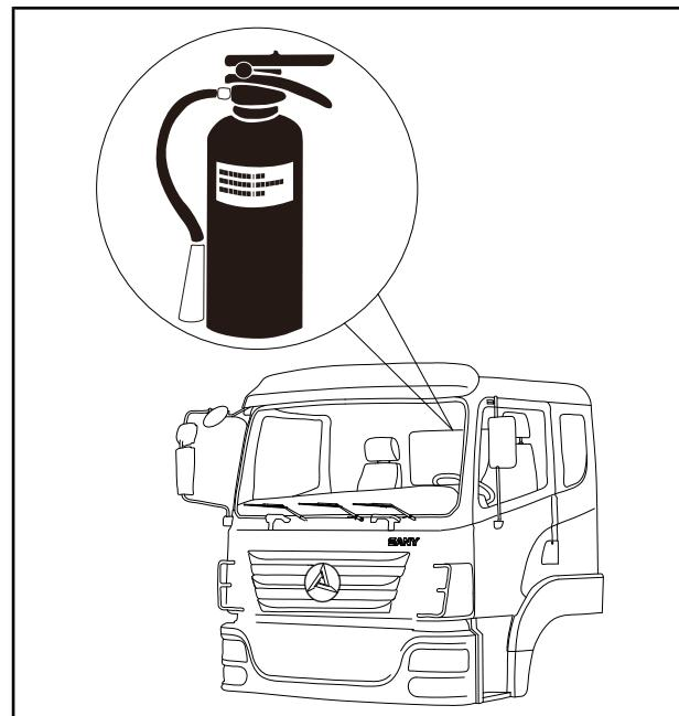
Fig.2-5 Location of fire extinguisher
