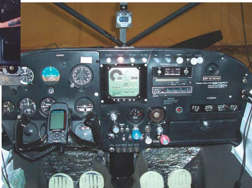
The new panel, equipped with Lowrance AirMap 500 GPS, VM-1000 engine management system, etc.
