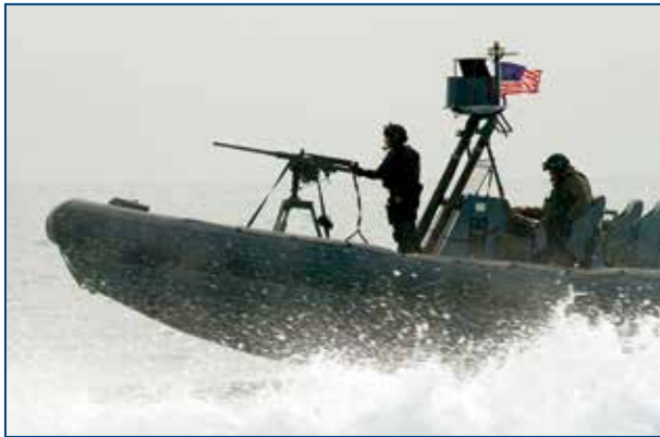
Naval Special Warfare Combatant-craft crewmen operate a Rigid-hull Inflatable Boat from a forward location. The RIB is equipped with M-2 .50-caliber machine guns.
