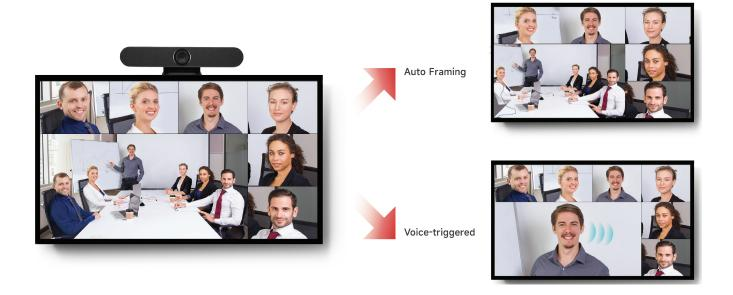
The function uses Al algorithms to automatically switch to multi-split screen layouts based on the number of participants, arranging close-ups of each participant. It also includes voice activation to switch between a panoramic view and a close-up of the speaker, providing an efficient communication experience.
