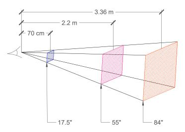
screen located at around 3.3m away from the viewer, the size of the wall-mounted screen should be around 84". These conditions are not always met in traditional meeting rooms, because either the screen is undersized or because some participants are sitting too far from the screen. When using a Silex PTE CoT system, all participants are seated at an equal distance from the screen and they all enjoy a perfect viewing experience.
