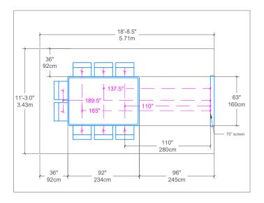
Room size required in a traditional setup using a 75" screen
