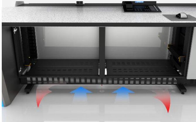
The ventilation air flow is arranged to enter through the bottom of the console. After the internal natural circulation, it is located on the desk according to the principle of exchange of air flow. The design of air holes can get a good heat dissipation effect.
