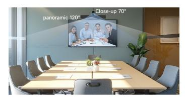
This system has a dual-camera design, featuring one ultra wide-angle camera and another 12x motorized PTZ close-up camera, both equipped with 4K UHD CMOS sensors for clear and detailed images. The panoramic camera has a 117° FoV, while the 12x PTZ close-up camera features a 70° FoV and 12x optical zoom, with a smooth motorized ±90° PTZ motor allowing to capture the smallest meeting details in large conference rooms.
