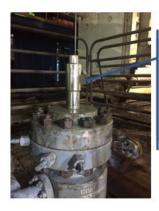
A 10K PSI Pack-Off is installed on the provided Nightcap Flange
