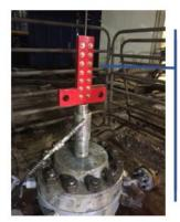
A compression style T-Clamp is installed on the antenna cable **above** the pack-off
