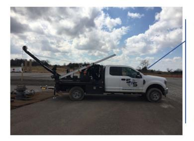
A 5 BY 5 Antenna Deployment Unit will arrive at your location. This specialized wireline deployment truck has been designed to use a minimal footprint with multiple styles of deployment. Whether we are able to back up over the wellhead and deploy via the boom or if your location requires remote tripod deployment the 5 BY 5 Antenna Deployment Unit is capable of getting the job done despite any onsite obstacles. Versatility and maximum safety is what the Deployment Unit was designed to achieve.
