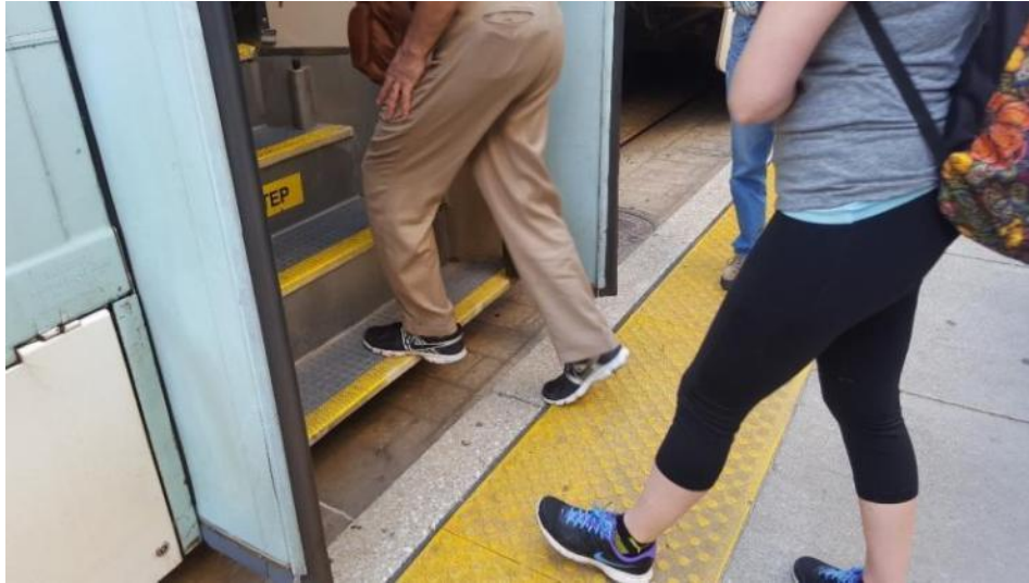
Figure 37: Stairs to enter Baltimore light rail vehicles further delay the system.
