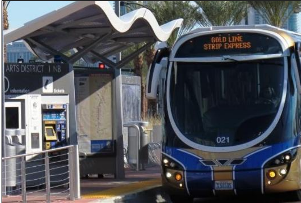
Figure 33: At-level boarding and off board fare collection on the Las Vegas BRT
