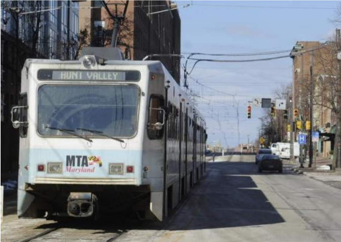
Figure 36: Left turns for mixed traffic are allowed across the Blue Line LRT tracks. BRT systems should restrict turns across the busway where possible.
