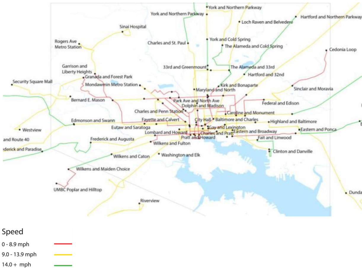
Figure 8: Average AM peak hour (8am – 9am) bus speeds on the top 20 Baltimore bus routes by ridership
