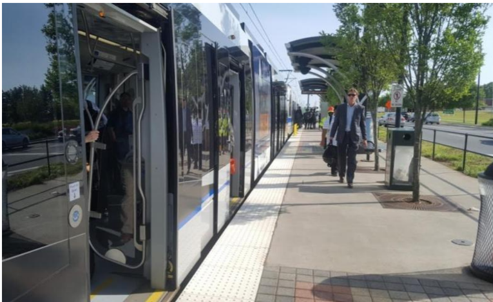
Figure 38: At-level boarding and off-board fare collection on the Charlotte LYNX light rail
