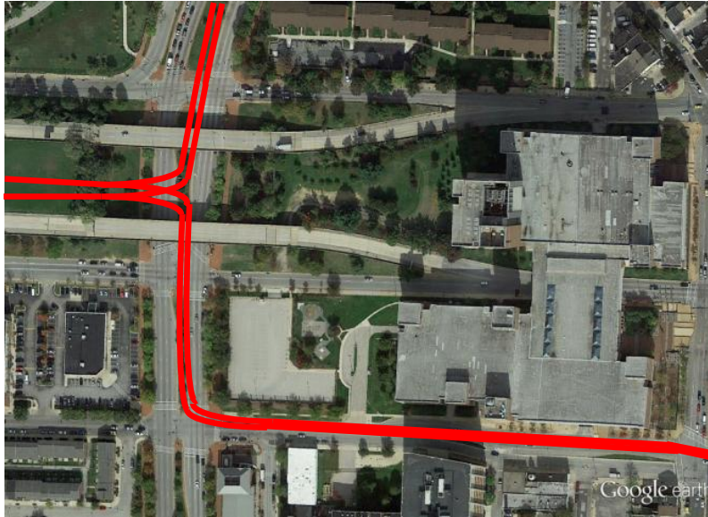
Figure 47: BRT could exit the median of Route 40 at MLK Blvd, use the median of MLK northbound and southbound turn immediately onto Saratoga Street.
