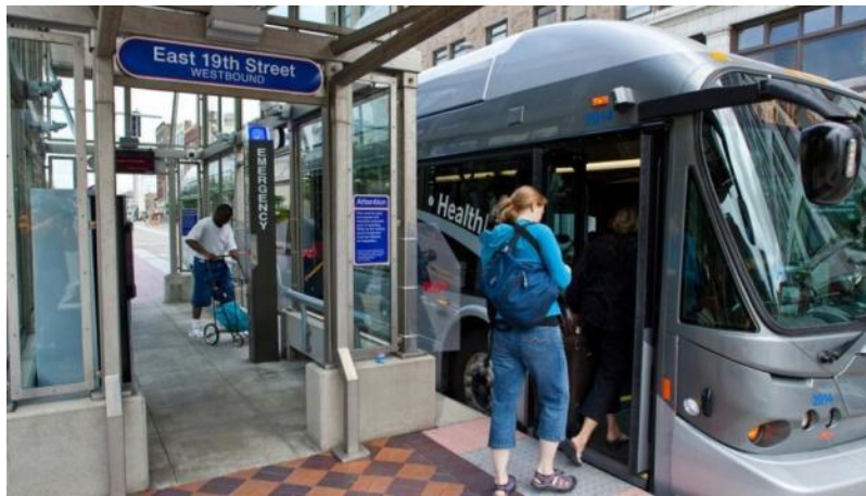
Figure 31: At-level boarding and off-board fare collection on the HealthLine BRT in Cleveland
