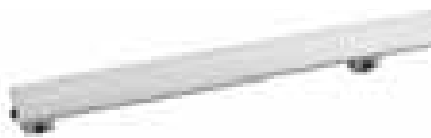
BA 65 Grate: Solid Stainless Steel (2 1/2" width, 3/4" height) - 7 Gauge 304L Stainless Steel Fits into XC 65, FC 65, FCS 65, FCB 65, FCH 65, OC 65, OCS 65, and OCH 65 channels.
