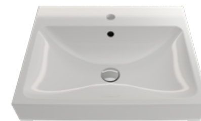
1077-XXX-012X Wall-Hung Sink 23-3/4" x 19" x 4" 41.09 lbs single-hole faucet setting (end code -0126); 3-hole faucet setting (end code -0127); with overflow; may be set on counter or used with metal console legs; NOT compatible with furniture base
