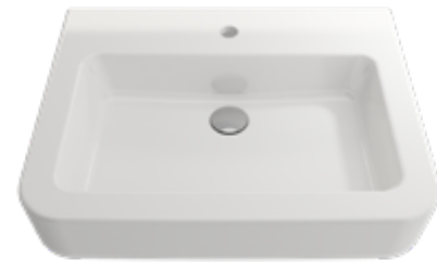
1123-XXX-012X Wall-Hung Sink 25-2/3" x 19-2/3" x 5" 47.02 lbs single-hole faucet setting (end code -0126); 3-hole faucet setting (end code -0127); with overflow (not pictured); may be set on counter or used with metal console legs
