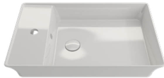
1479-XXX-0126 Vessel Sink 23-1/2" x 15" x 4-1/2" 24.47 lbs single-hole setting; with overflow; comes with a color-matched, pop-up drain cover
