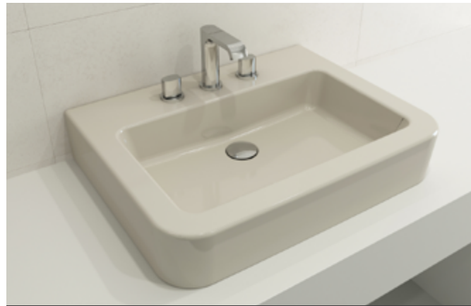
1123-XXX-012X Wall-Hung Sink 25-2/3" x 19-2/3" x 5" 47.02 lbs single-hole faucet setting (end code -0126); 3-hole faucet setting (end code -0127); with overflow (not pictured); may be set on counter or used with metal console legs
