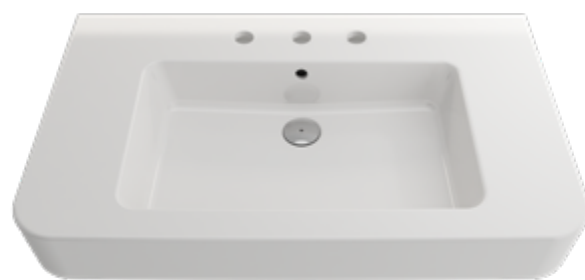
1124-XXX-012X Wall-Hung Sink 33-2/3" x 19-2/3" x 5" 58.07 lbs single-hole faucet setting (end code -0126); 3-hole faucet setting (end code -0127); with overflow; may be set on counter or used with metal console legs
