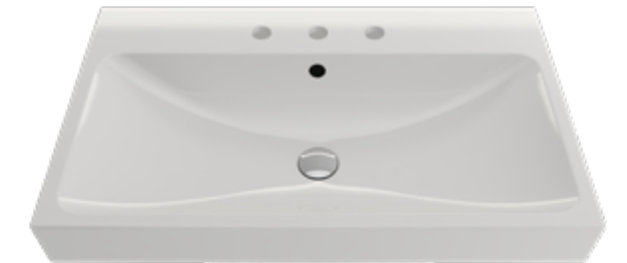
1078-XXX-012X Wall-Hung Sink 31-1/2" x 19" x 4" 51.92 lbs single-hole faucet setting (end code -0126); 3-hole faucet setting (end code -0127); with overflow; may be set on counter or used with metal console legs; NOT compatible with furniture base
