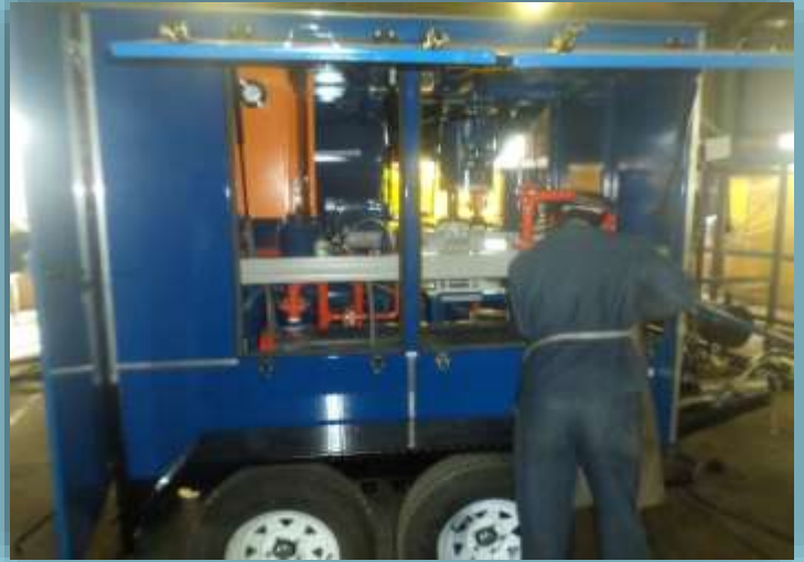
Nirvana Substation - oil circulation (40 MVA, 88/11 Kv)
