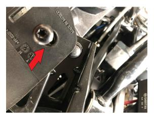
Once the 2 lower bolts are removed proceed to removing the hood & front end cover.
