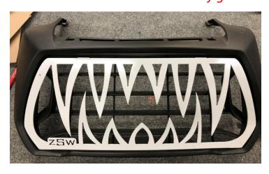
Ensure the lower tab sits flush with the inner edge of the grille. You may need an extra hand to help flex the grille to the contour of the factory front end so the tab sits flush.
