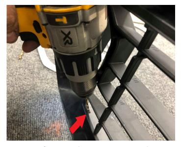
Note: Take your time as you are going to have to drill at a slight angle and don't want to drill a bigger hole then needed.
