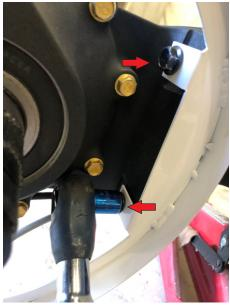
After you have tightened the two swing arm bolts, secure the bottom tab of the wheel ring with the supplied zip tie to the bottom factory hole as shown in the picture.
