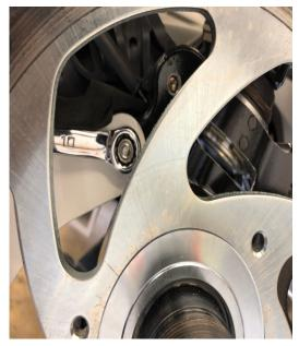
After you are done tightening proceed to the opposite side to complete the front installation. Complete the front by placing the front wheels back on.
