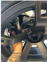
Set the caliper down and remove the two bolts as shown.
