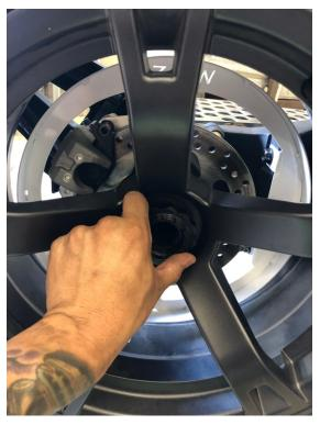
Note: Each wheel ring has spots open to allow for zip ties to be used if needed.
