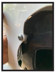
Adjust rear tab accordingly to align to mounting hole. Adjustment can be made by hand. Add (1) 1/4" washer and stock bolt. After you align the belt guard, tighten all bolts in place.
