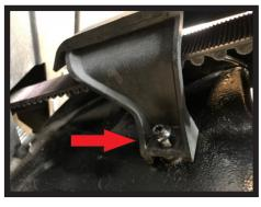
Start assembly by hand tightening and adding (2) 1/4" washers for the front bottom bolt and (2) 1/4" washers for the top bolt.
