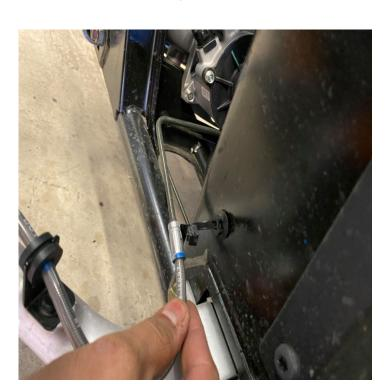
Next slide the driver side plate in at an angle around the brake line. Note: The brake line may need to be moved slightly or bent to get the plate in. After the plate is in place, install the bolts (bigger bolts go on top and smaller ones on the bottom).
