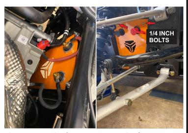
Start the installation by identifying the driver and passenger side plates. Passenger side plate is for the jump ports. The larger 1/4 inch bolts and nuts go into the upper side of the plate. The smaller 3/16 bolts go into the lower side of the plate.
