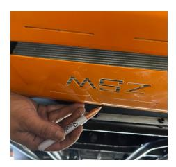
To install, align the Front Lower Accent Skid Plate to the bike and mark all the holes for drilling reference.
