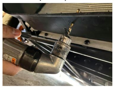
Lastly, install the (4) 1/4 inch bolts towards the front of the bike. Then install the (3) 3/16 smaller bolts towards the back by the factory air dam, for the 3/16 bolts use a bottom and top washer.
