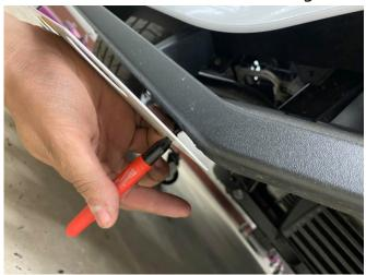
After the holes are drilled install the hardware provided. Place the washer on the top side of the inner lip under the nut.
