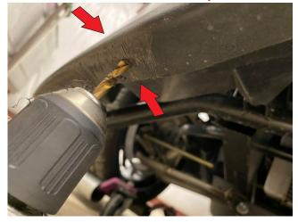
Once you have aligned the splitter, begin marking the drill holes. Start with the hole towards the center of the Slingshot.
