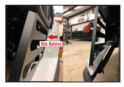
After the grille is aligned and looks good proceed to drill the 3 holes with a 1/4 inch drill bit.
