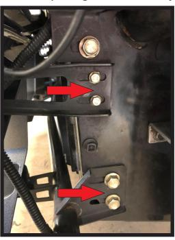
**Note:** Some front bumpers might need to be adjusted and aligned for the fillers to fit perfectly . We have noticed some SS bumpers have some variations on fitment from the factory specs, so please keep that in mind. Bumper may need to be adjusted if the fit is too tight.
