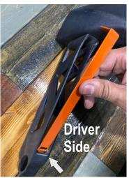
To install, slide the arm trim towards the bottom of the mirror canal as shown.
