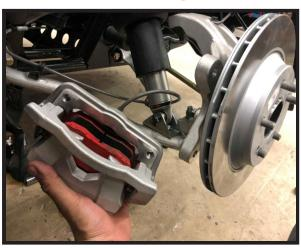
Next place the caliper in a safe spot then remove the rotor.
