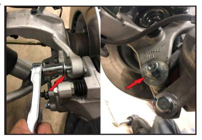
After you have removed the caliper bolts, remove the caliper itself.
