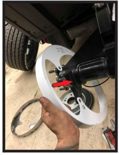
Pass the caliper through the ring just like in Figure 1 and 2 from Step 5. Re-install the rotor and the brake caliper. Then proceed to line up the wheel ring with the caliper bolts. Continue to tighten the caliper bolts back to factory specs  $60\pm3$  ft-lb (81 $\pm4$ Nm)
