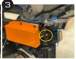
For 2017+ models use 10mm lock nut and tighten side arm onto the stock bolt. Insert plastic push clips into head light back cover.
