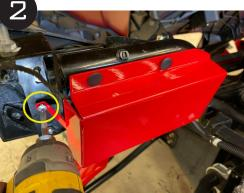
Insert plastic push clips into head light back cover. For 2015-2016 models use self tapping screws to secure side arm.
