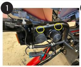
To install, remove factory zip tie to loosen wires. Remove factory plastic clips from back of bar.
