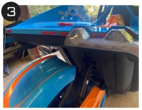
Ensure the bonding surface is clean, dry and free of any product contamination where the 3M will be applied to the bike. With the supplied 3M cut into sections as shown in the picture above and begin to apply it to the bike.
