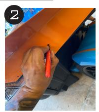
After the spoiler has been test fitted on both sides, begin marking the holes where they will be drilled.
