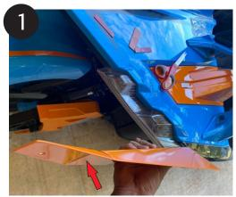
Start off by getting the spoiler and test fitting it to the bike. Notice: There is a relief cut that is on each spoiler. Bend and form the spoiler as much as possible to the curve of the bike where the spoiler will be installed.
