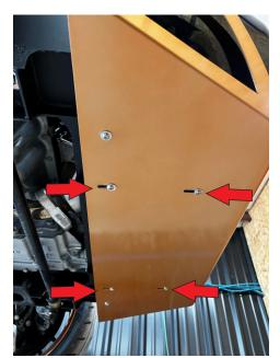
Now tighten the factory rear brackets with the factory bolts that were removed on Step 3
