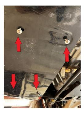
Look towards the rear where the factory bolts were removed and remove the factory plastic lower nut retainer on the 2 back side bolts only.
