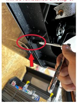
Now hold new front splitter and position in place, install 2 of the 1/4" new bolts towards the front side of the splitter and hand tighten.
