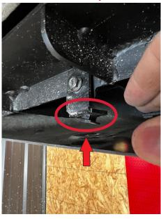
Next, remove the 2 back brackets the plastic nut retainers were attached to. Note: Save the 2 factory bolts as they will be reinstalled on Step 6.
