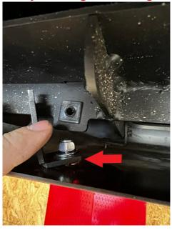
Adjust lower splitter to desired depth, slots shown allow for adjustment.
