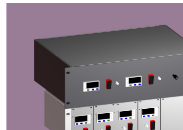
HSLM shown in rack-mount system along side four HCM's (heater control modules).
