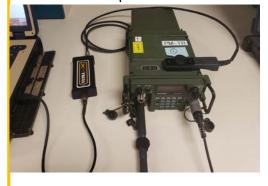
The ULTRALink offers the latest in technology innovations with a Field Programmable Gate Array (FPGA) design. A fully implemented IP stack supporting UDP/TCP data packages to Tactical radio.
