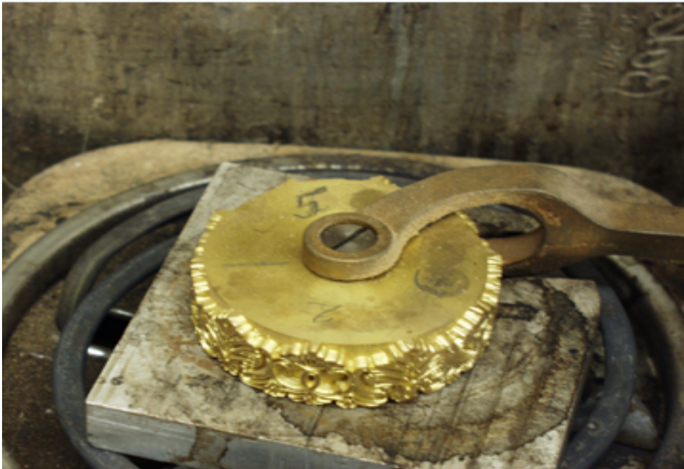
Tool with registration marks. Note aluminum heat sink.
