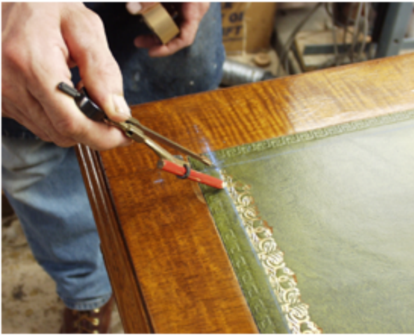
Marking for laying out the miter.
