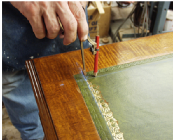
Marking for laying out the miter.
