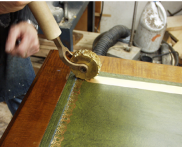
Note the failed impression. This will be fixed later.
