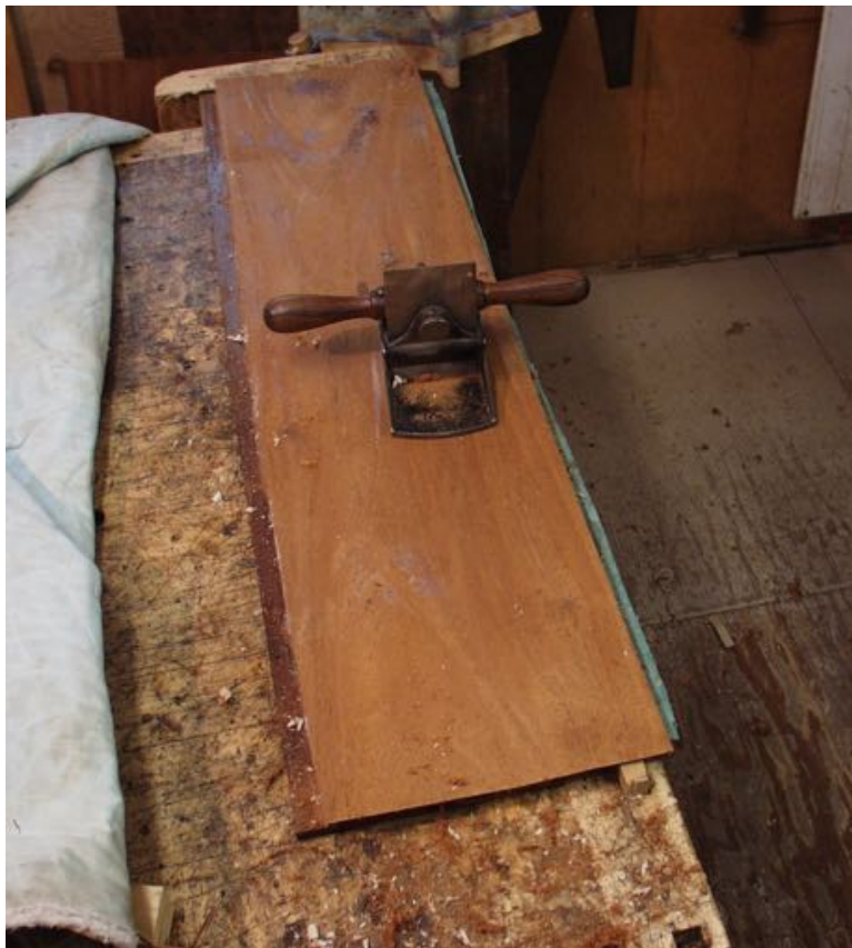
Surfacing and leveling veneer. Overhang trimmed after.
