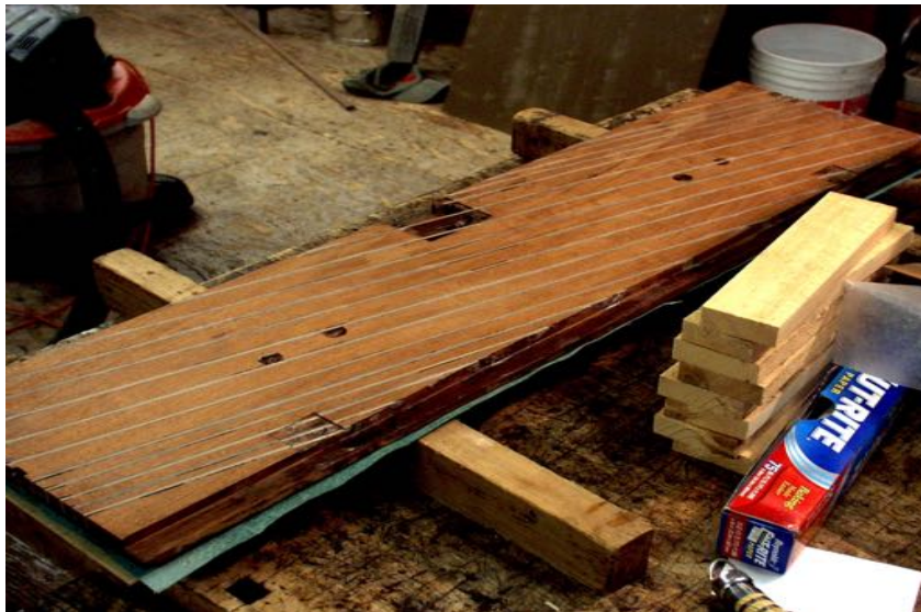
Kerfing procedure completed with extra set of splines near corners.
