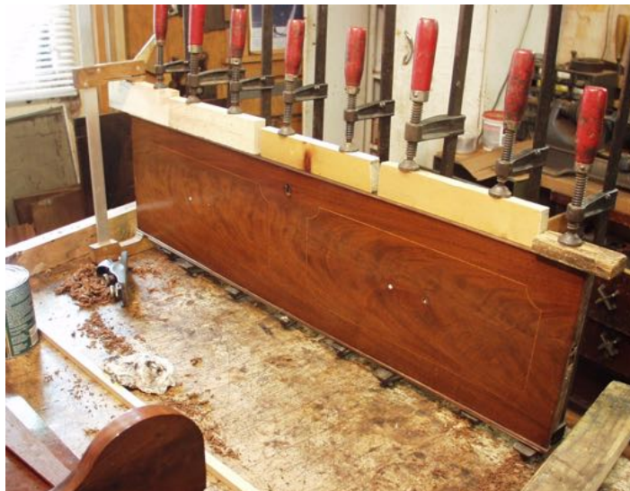
Cock-bead being glued on top and bottom first.
